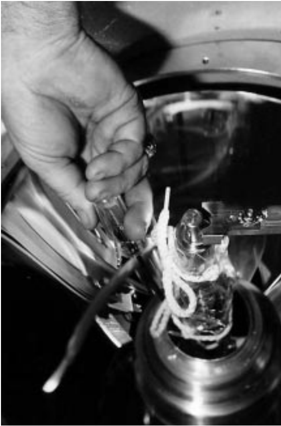
5. Using extended Hex-Driver, Tighten Rear Lamp Clamp.
