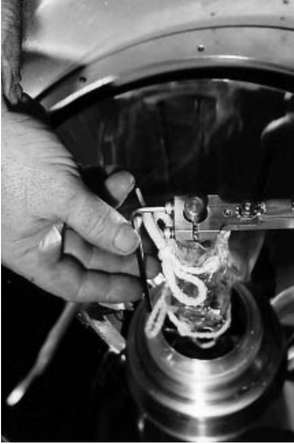
6. Reinstall Top Portion of Front Lamp Clamp.
