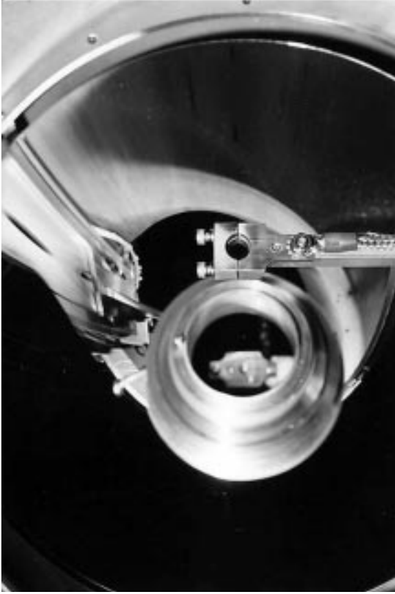
2. Optical Assembly Prior to Lamp Installation
