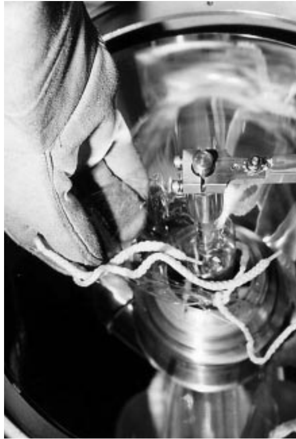
7. Carefully Remove Flexible Shield from Lamp.
