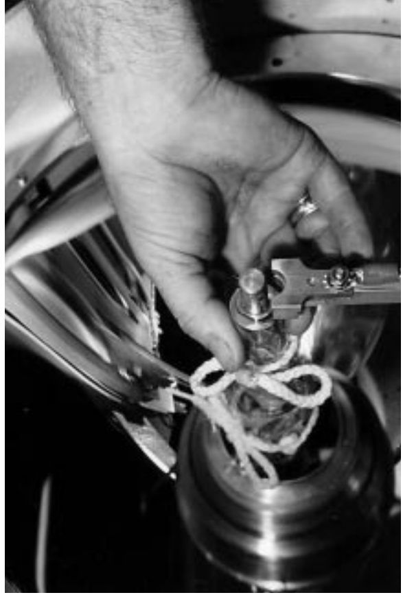
4. Insert Screw and Lamp onto Rear Lamp Mount until Seated.
